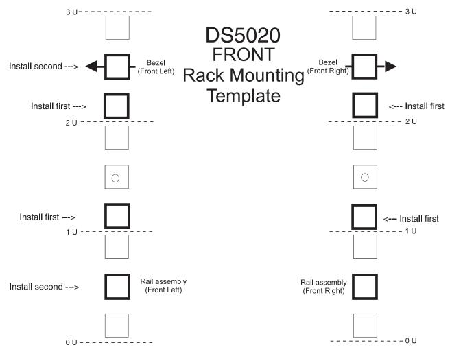
Figure 89. Front rack mounting template
